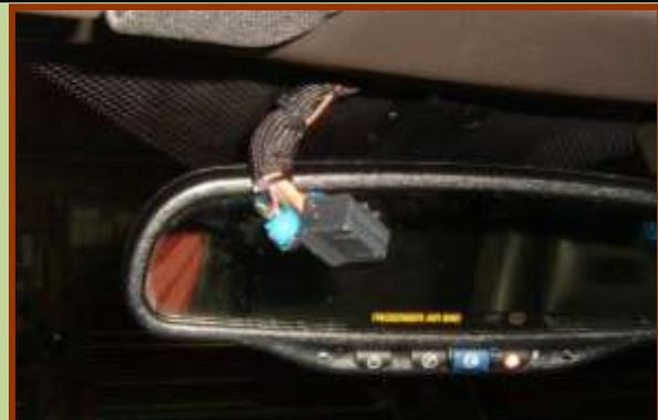
For a C6 Corvette with auto-dim, the Pink wire, lower center, is +12V and the Black wire, top row is ground. For C6 without the auto-dim mirror the Orange wire in the top row is +12V and the Black wire, top row, is ground.
