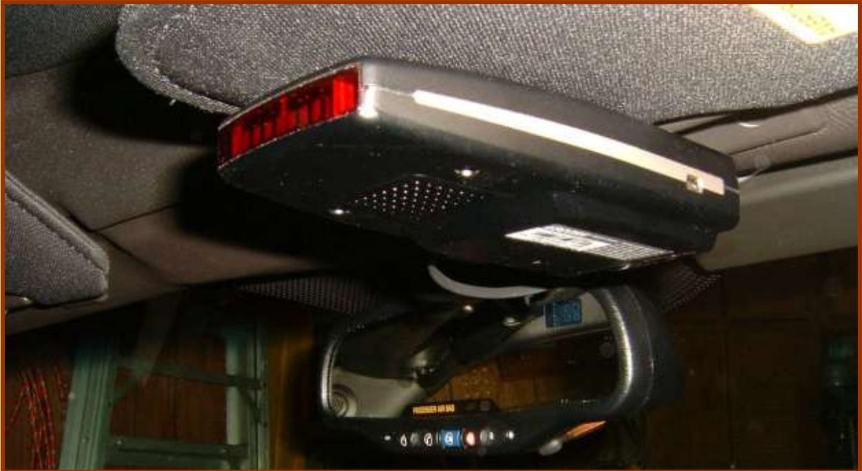
If you want your radar detector out of the way, the best place to install it is with a clip on the passenger visor. The added benefit of that location is you can easily connect to the 12V power available at the mirror. Power is only on when the car is running. (On my '93 Vette spliced into the visor mirror light but this was easier.) If you use the cigarette lighter and a windshield mount the power is always on and if you leave connected for a week a dead battery might greet you!
